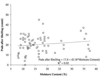
Fig. 2. Comparison moisture content and unshelled pod count for shelling with the grade sheller without pod recycling.
