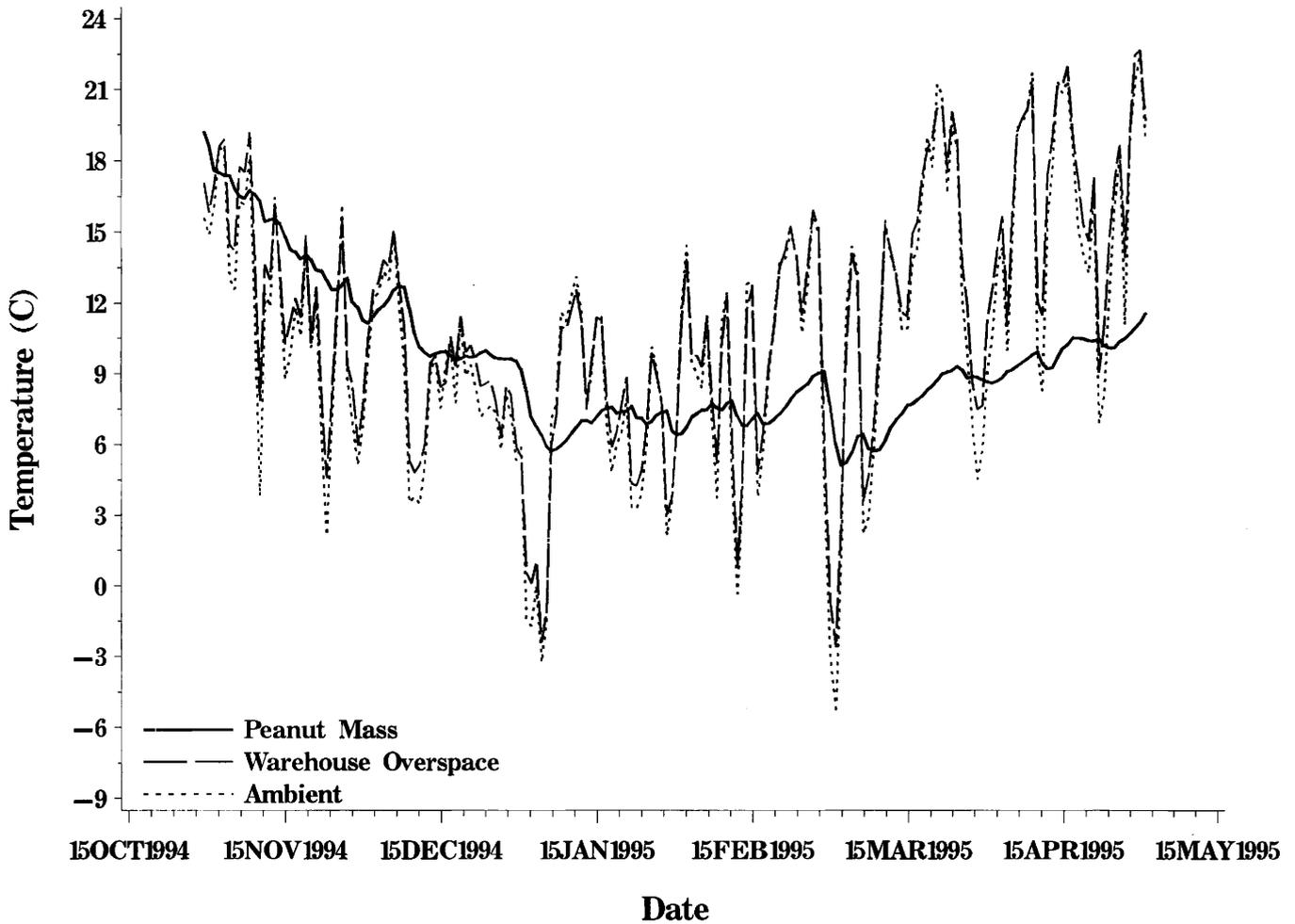
Fig. 2. Mean daily temperatures of the peanut mass, warehouse overspace, and ambient conditions during storage of farmer stock peanuts in an aerated warehouse in west Texas during the 1994-95 storage period.
