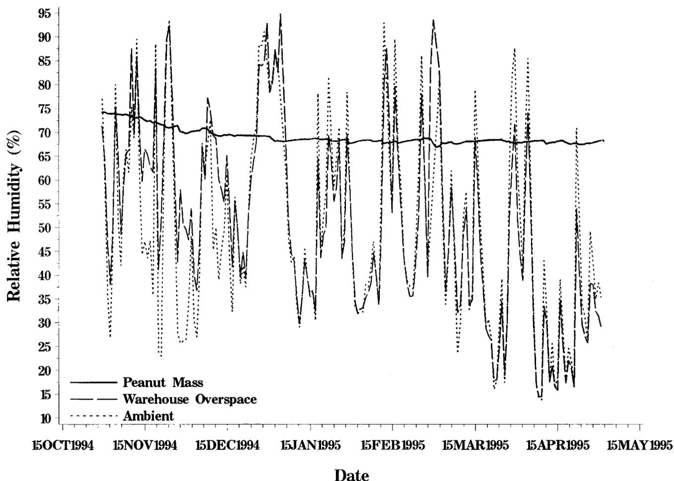
Fig. 4. Mean relative humidity of the peanut mass, warehouse overspace, and ambient conditions during storage of farmer stock peanuts in an aerated warehouse in west Texas during the 1994-95 storage period.
