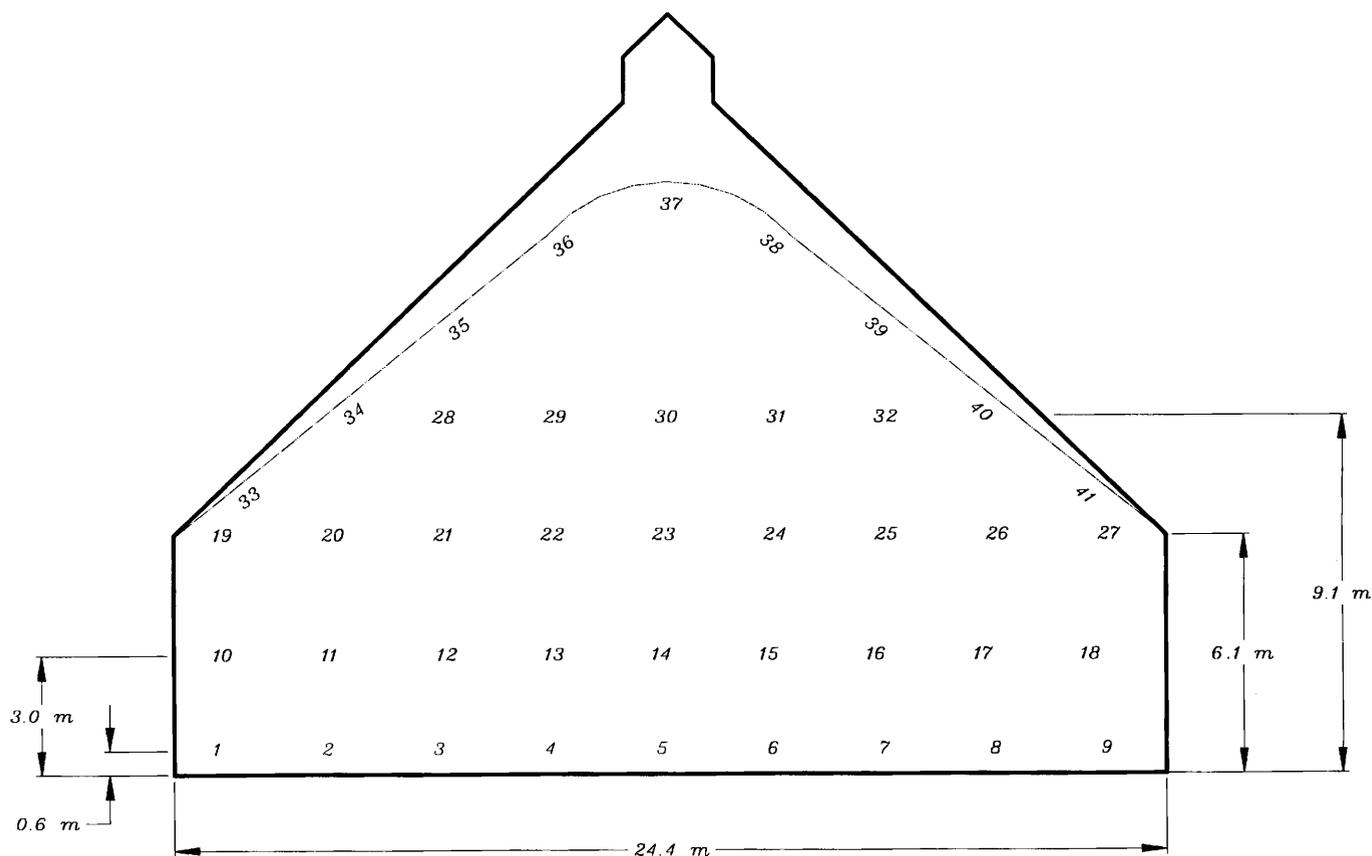
Fig. 1. Cross section of warehouse indicating numbered sensor and sample locations within the peanut mass.
