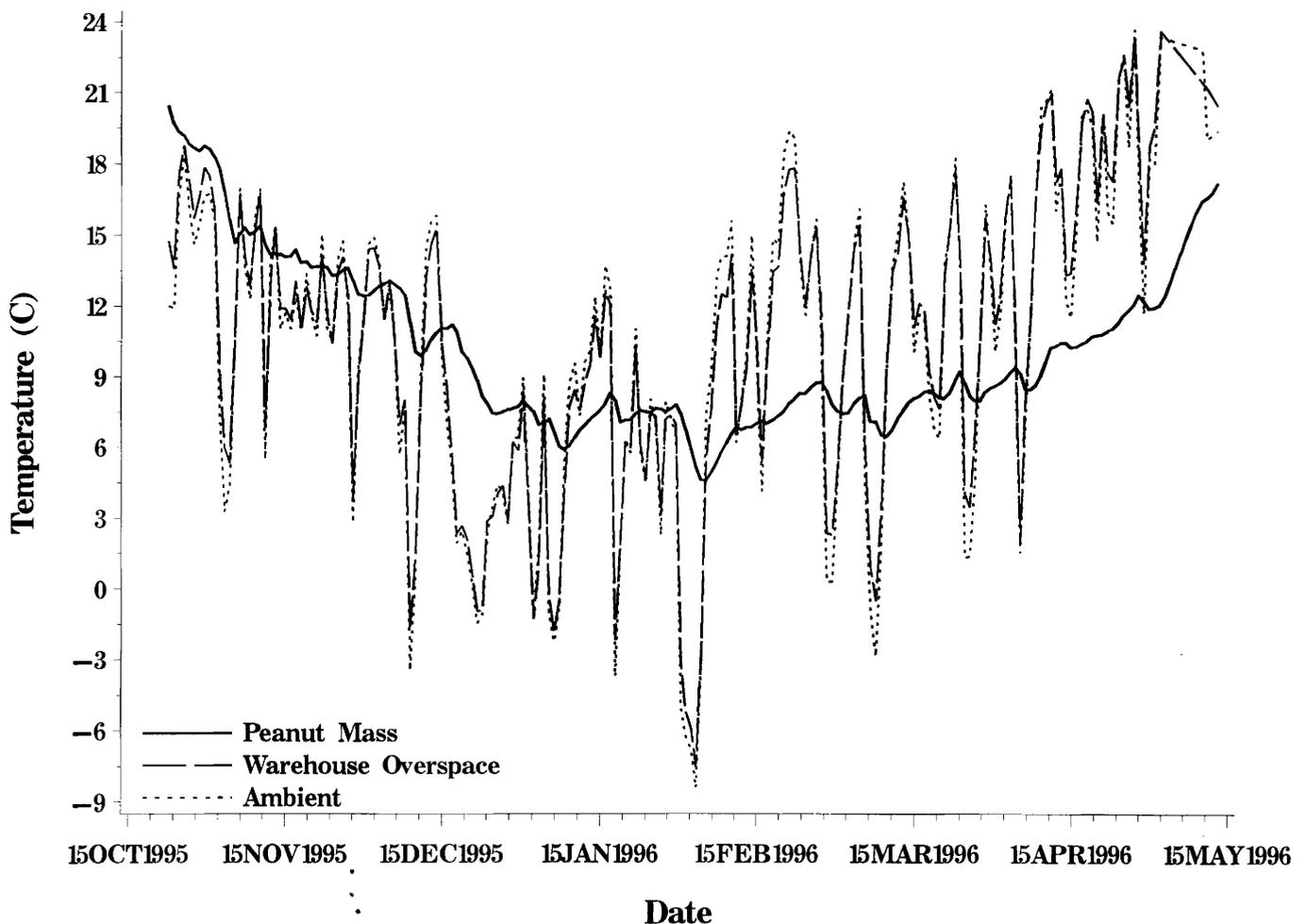
Fig. 3. Mean daily temperatures of the peanut mass, warehouse overspace, and ambient conditions during storage of farmer stock peanuts in an aerated warehouse in west Texas during the 1995-96 storage period.
