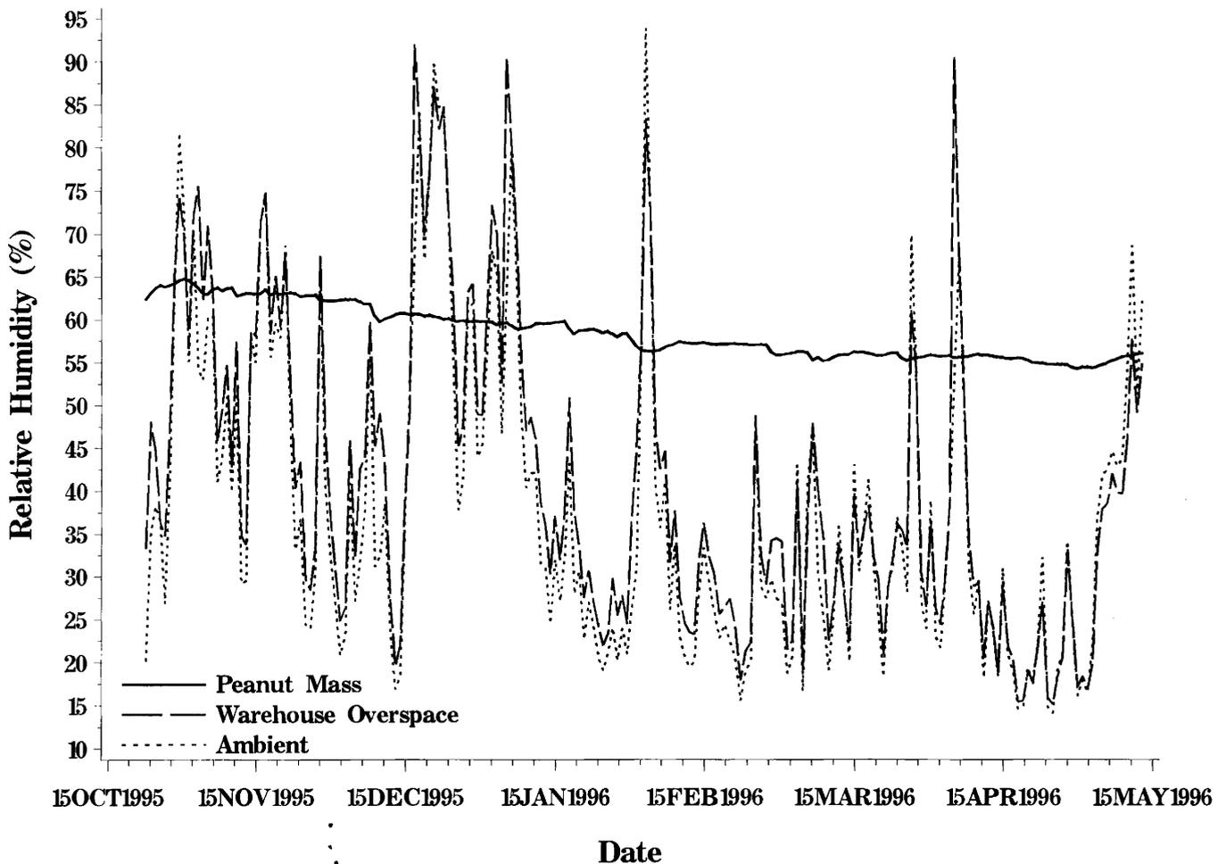
Fig. 5. Mean relative humidity of the peanut mass, warehouse overspace, and ambient conditions during storage of farmer stock peanuts in an aerated warehouse in west Texas during the 1995-96 storage period.
