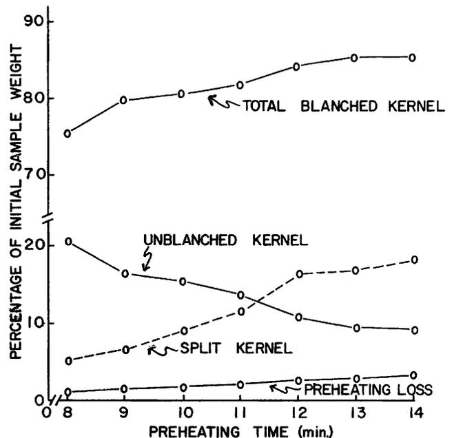
Fig. 7. Total blanched kernels, unblanched kernels, split kernels, and preheating loss versus preheating time for medium Florigiant seed (initial mc — 6.4%, blanching time — 90 sec, input air pressure — 17.6 psi).
