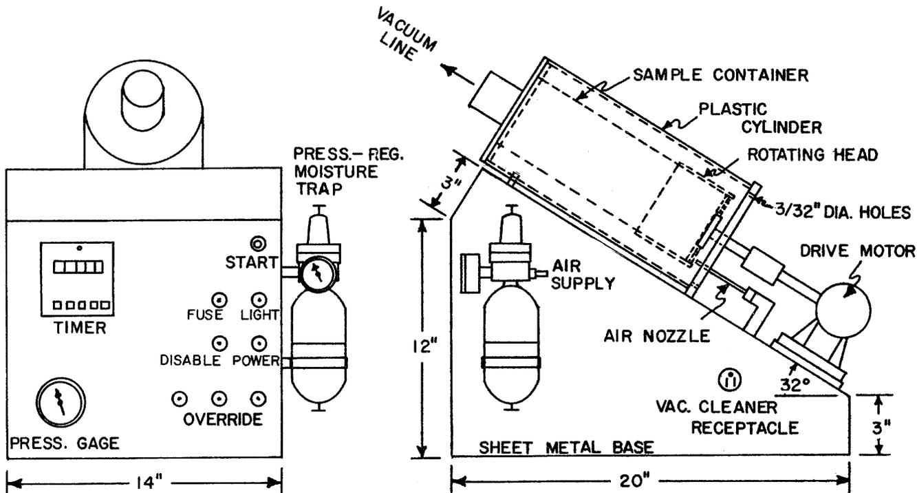
Fig. 2. Schematic of laboratory blanching device.
