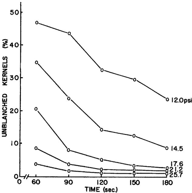
Fig 5. Percentage of unblanched kernels versus time at five pressure settings for the laboratory blanching device.
