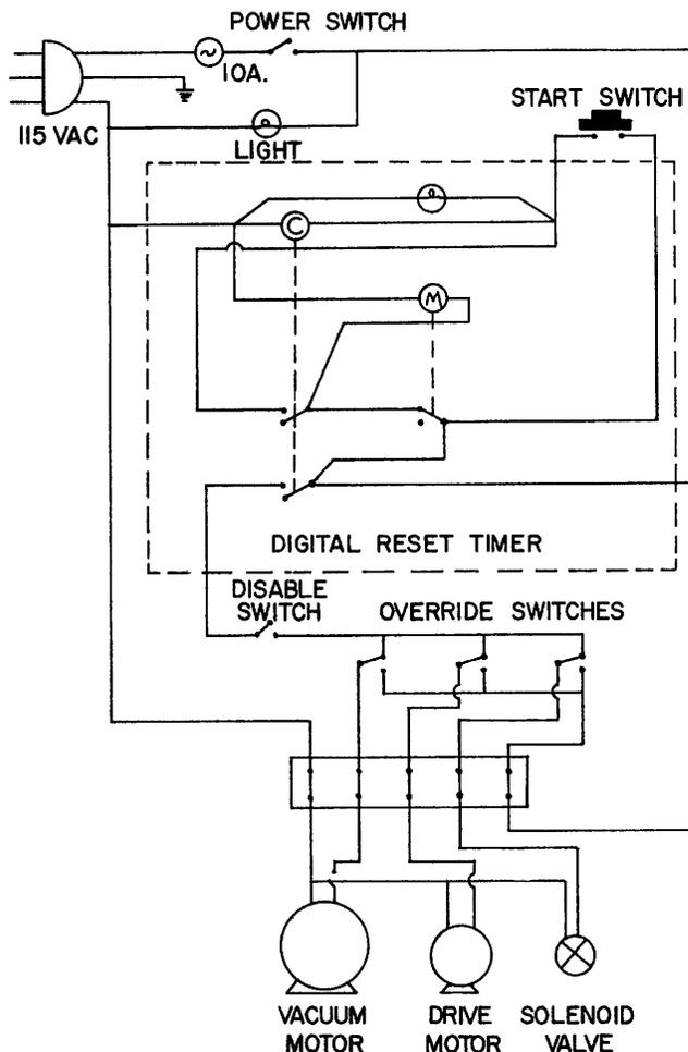
Fig. 3. Wiring schematic for laboratory blanching device.
