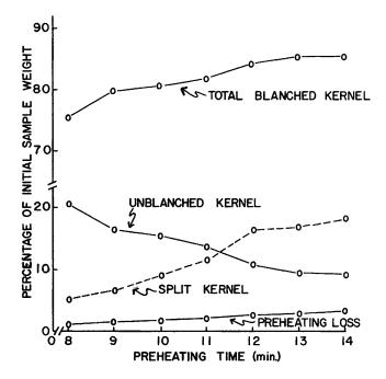
Fig. 7. Total blanched kernels, unblanched kernels, split kernels, and preheating loss versus preheating time for medium Florigiant seed (initial mc - 6.4%, blanching time - 90 sec, input air pressure - 17.6 psi).
