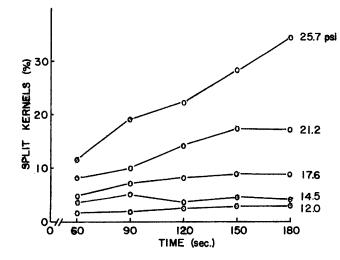
Fig. 4. Percentage of split kernels versus time at five pressure settings for the laboratory blanching device.
