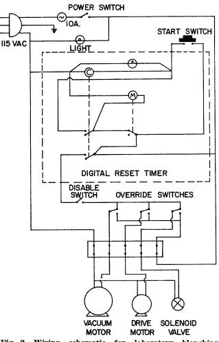
Fig. 3. Wiring schematic for laboratory blanching device.
