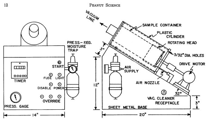
Fig. 2. Schematic of laboratory blanching device.
