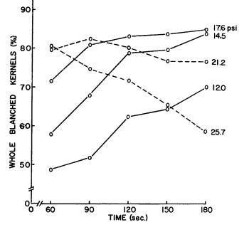
Fig. 6. Percentage of whole blanched kernels versus time at five pressure settings for the laboratory blanching device.
