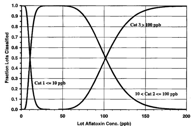
**Fig. 4. Fraction of lots classified into three categories when measuring loose shelled kernels taken from a 50-kg farmers stock sample and using dual tolerances of 10 and 100 ppb.**
