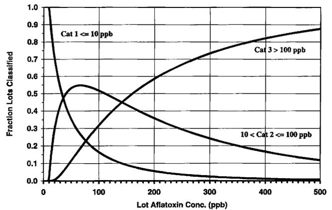
**Fig. 3. Fraction of lots classified into three categories when measuring loose shelled kernels taken from a 2-kg farmers stock sample and using dual tolerances of 10 and 100 ppb.**
