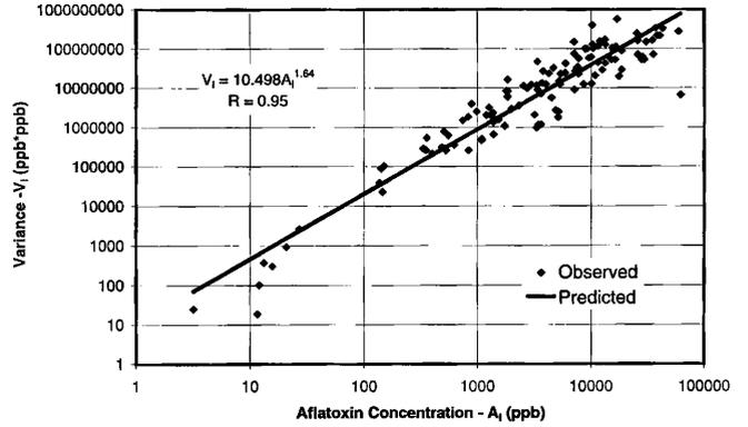
Fig. 2. Full log plots of variance ( $V_1$ ) versus aflatoxin when measuring aflatoxin ( $A_1$ ) among loose shelled kernel samples.
