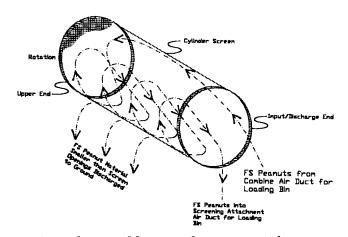
Fig. 2. A schematic of farmer stock peanut material movement during trommel operation.
