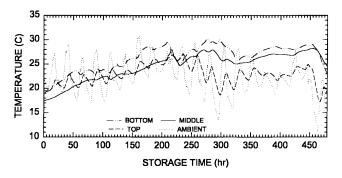
Fig. 4. Average hourly temperatures for the top (30 cm), middle (76 cm), and bottom (120 cm) depths in box 6 with the ambient temperatures for the 1995 storage season.
