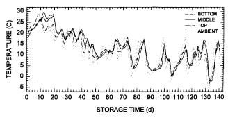
Fig. 5. Average daily temperatures for the top (30 cm), middle (76 cm), and bottom (120 cm) depths in box 6 with the ambient temperatures for the 1995 storage season.
