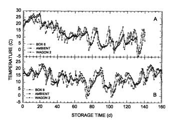
Fig. 6. Average daily temperatures for the middle depth (76 cm) of box 6 and wagon 2 with the ambient temperatures for the 1995 (A) and 1996 (B) storage seasons.
