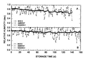
Fig. 7. Average daily relative humidity for the middle depth (76 cm) of box 6 and wagon 2 with the ambient relative humidities for the 1995 (A) and 1996 (B) storage seasons.
