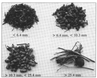
Fig. 2. Typical separations from the triple deck, parallel belt screen deck gaps.
