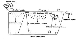
Fig. 1. Schematic of the triple deck, parallel belt screen.
