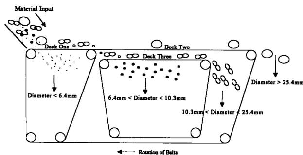
Fig. 1. Schematic of the triple deck, parallel belt screen.
