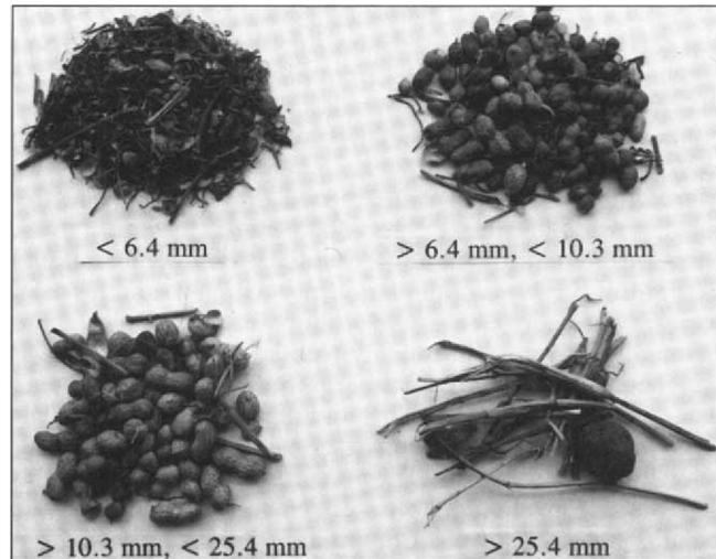
Fig. 2. Typical separations from the triple deck, parallel belt screen deck gaps.
