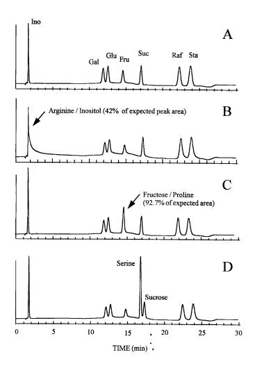
Fig. 1. Sugar standards and interfering amino acids.
