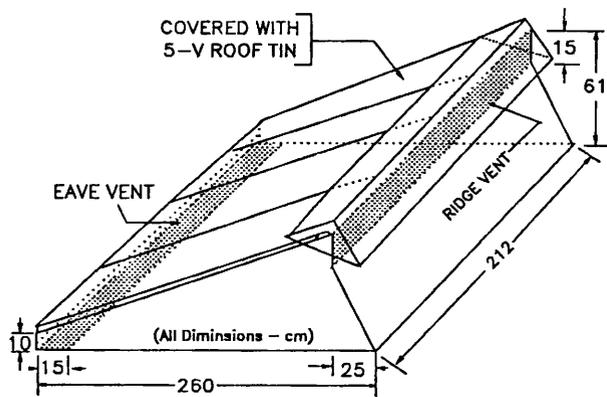
Fig. 1. Shed cover for half-trailer container.
