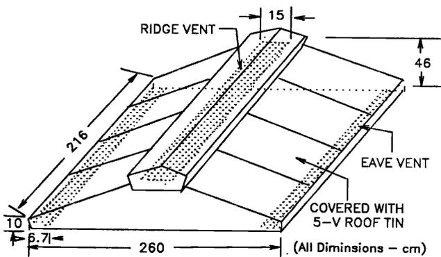
Fig. 2. A-frame cover for half-trailer container.
