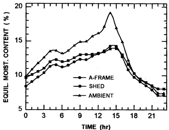
Fig. 3. Headspace and ambient equilibrium moisture content for containers with a shed and A-frame type cover (14 Nov. 1993).
