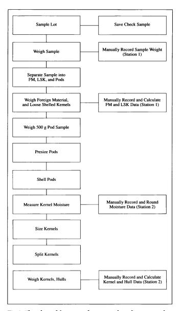
Fig. 1. Flow chart of the current farmers stock grading process that includes a manual data collection system. The sample from the lot includes foreign material (FM) and loose shelled kernels (LSK).
