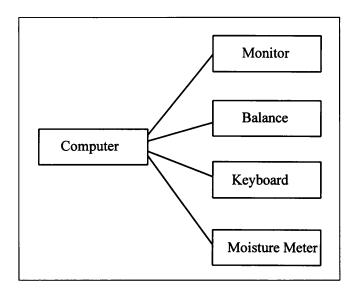
Fig. 5. Diagram of the automated data collection system developed for an automated grade sample cleaning, shelling and sizing system.
