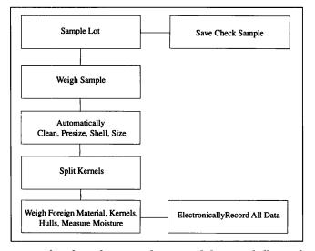
Fig. 4. Flow chart of a proposed automated cleaning, shelling and sizing system that includes an automated data collection system.
