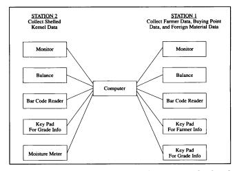
Fig. 3. Diagram of the automated data collection system developed for current grading rooms.
