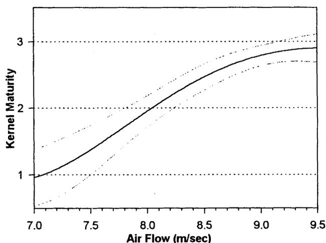
Fig. 4. Regression analysis between kernel maturity and air flow ( $\text{m/sec}$ ) required to float Florunner peanut pods. Kernel maturity of 1=immature, 2=mid-mature, and 3=mature. 95% confidence interval shown.  $R^2=.55$ .
