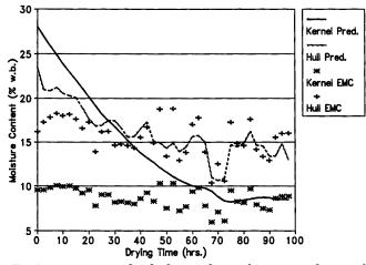
Fig. 3. Drying curves for the bottom layer of wagon number 21 of the 1989 drying experiments.
