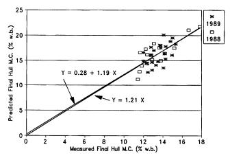
Fig. 11. Comparison of predicted and measured final hull moisture contents at top of peanut wagons during 1988 and 1989.
