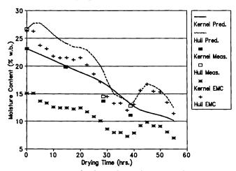
Fig. 6. Drying curves for the top layer of wagon number 46 of 1989 drying experiments.
