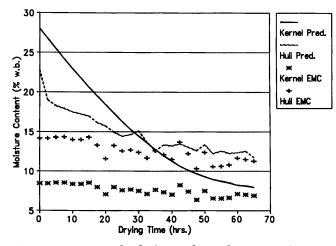
Fig. 1. Drying curves for the bottom layer of wagon number 11 in 1989 experiments.
