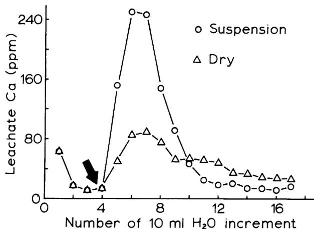
Fig. 1. Effect of 2 methods of applying gypsum on the leachate Ca concentration after applying increments of water. Gypsum applied at arrow just prior to 4th increment. Values are averages from duplicate analyses from 3 soils.
