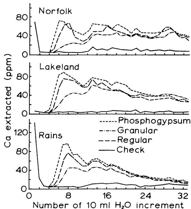
Fig. 2. Calcium leaching rate by increments of water on 3 soils with and without the application of 3 calcium sulfate sources.
