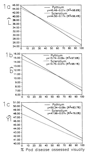
Fig. 1. Linear regression between colorimeter values and percent pod disease determined visually for Pythium and Sclerotium infected samples. 1a = Hunter color value L, 1b = Hunter color value b, and 1c = Yellowness Index. Mean of five determinations at each infection class was regressed on infection class (0%-100%). Pods were hand selected to approximate the eleven infection levels.
