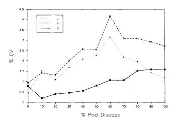
Fig. 2. Coefficients of variability in colorimeter reading at each of eleven visually-determined pod disease levels for a Pythium infected sample. L and b are Hunter color values; YI is a yellowness index. CV was calculated based on five measurements at each infection level. Pods were hand selected to approximate the eleven infection levels.
