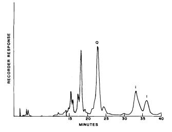
Fig. 2. Chromatogram of Spanwhite skin extract. (Flow rate 2 ml/min, 10 min linear gradient [90-65% of 1% HOAC and 10-35% of methanol] on a 30 cm X 3.9 mm  $\mu$  Bondapak C<sub>18</sub> column). Q = quercetin derivative; I = isorhamnetin derivative.
