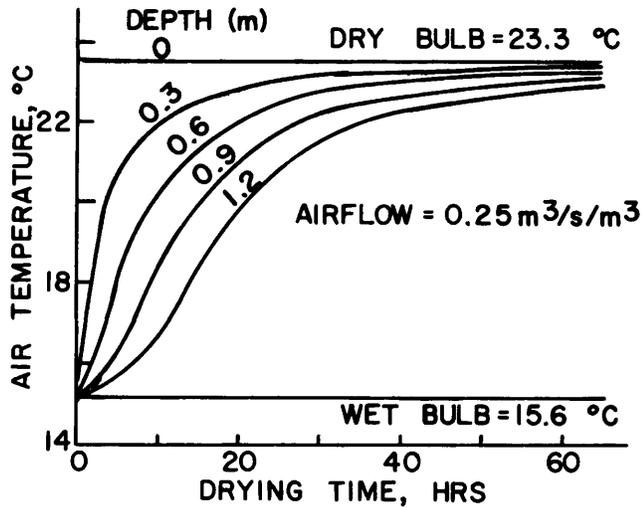
Fig. 2. Air temperatures with time at selected depths in a fixed-bed, controlled-temperature peanut drier as peanuts dried from a moisture content of 30% to 8.2%.
