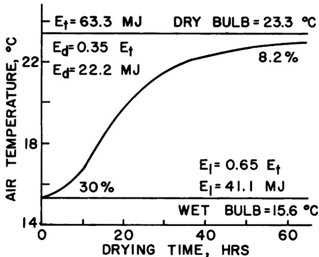
Fig. 3. Graphic representation of total energy input with time for fixed-bed drying of conventionally harvested peanuts from 30% moisture content to 8.2%.
