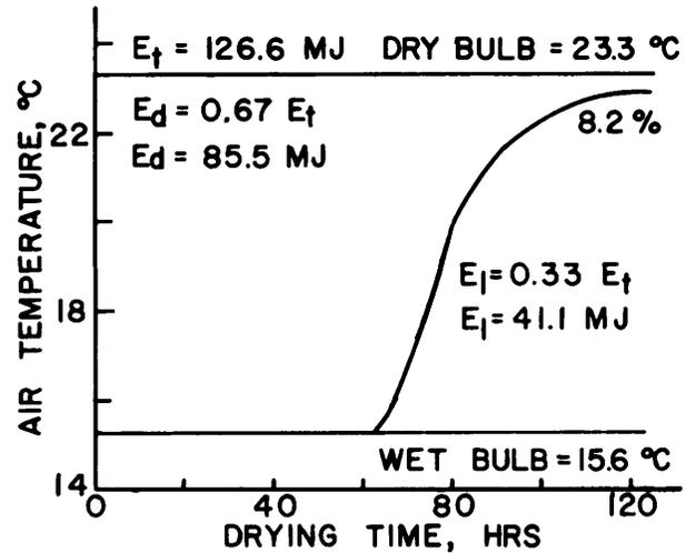
Fig. 4. Graphic representation of total energy input with time for fixed-bed drying of direct harvested peanuts from 55% moisture content to 8.2%.
