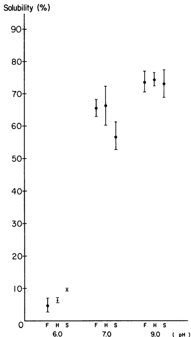
**Fig. 1. Effect of moist heat treatment (107°C for 20 min.) and storage at 24°C on solubility (%) of FD peanut protein preparations. Results are expressed as means ± standard deviation, F=fresh, H = moist heat, S = 18 mo storage.**
