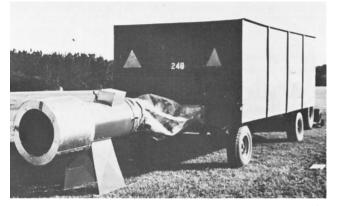
Fig. 2. Muffler mounted on inlet of fan-burner unit in position for SPL tests.
