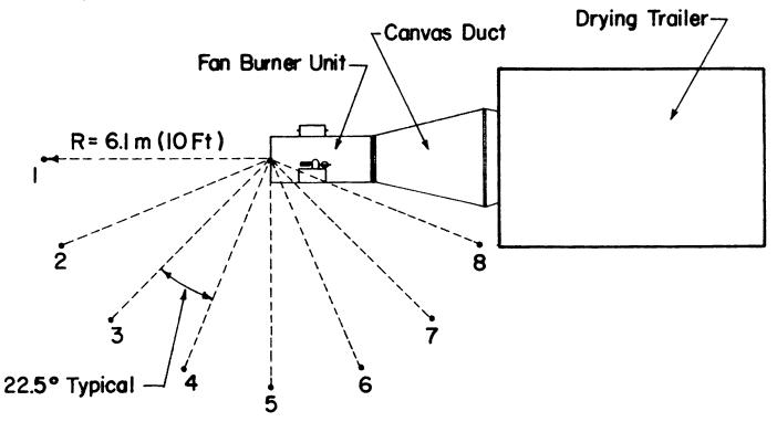
Fig. 1. Location of measurement positions for SPL tests.
