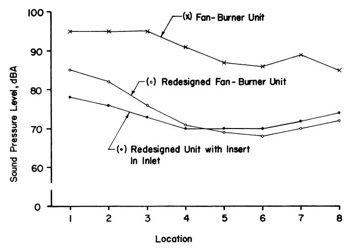
Fig. 6. Sound-pressure levels with redesigned fan housing with and without insert in inlet.
