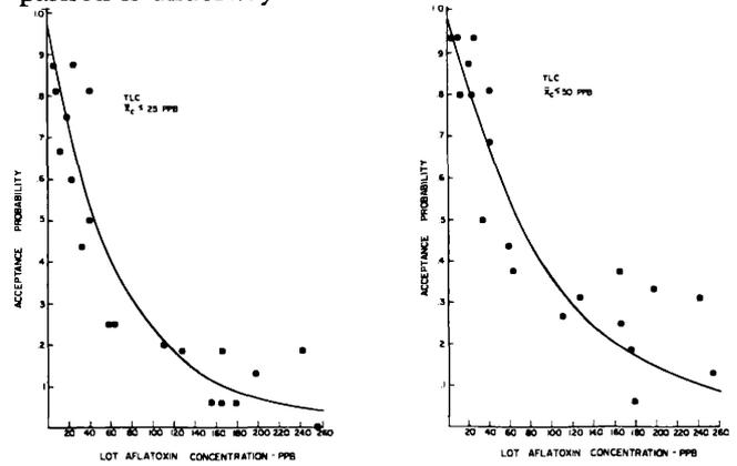
Fig. 3. (left) Observed and predicted acceptance probabilities associated with the TLC method, 465-g sample, and 25 ppb critical level.
