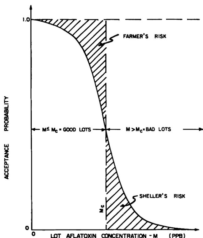
Fig. 1. Typical operating characteristic (OC) curve for evaluating sampling plans.
