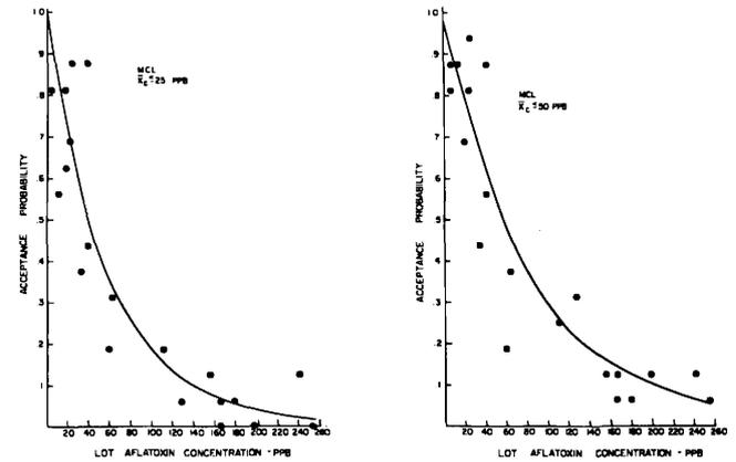
Fig. 5. (left) Observed and predicted acceptance probabilities associated with the minicolumn method, 465-g sample, and 25 ppb critical level.
