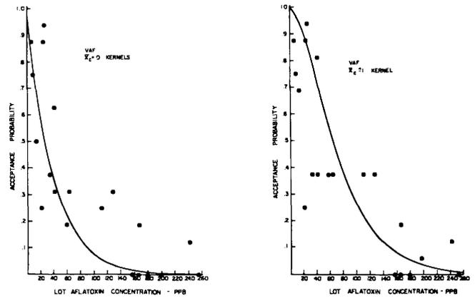
Fig. 7. (left) Observed and predicted acceptance probabilities associated with the visible *A. flavus* method (VAF), 465-g sample, and a critical level of 0 VAF kernels.
