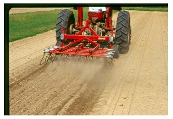
Fig. 3. The initial cultivation with a tine weeder must be prior to weed and crop emergence. Peanut seedlings are beginning to 'crack' the soil surface in the row on the right side of this picture, which allows for maximum aggressiveness, with little risk of peanut injury.
