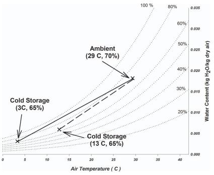
Fig. 1. Psychrometric chart showing thermodynamic properties of air as it transitions from ambient conditions (29 C, 70% relative humidity) to typical cold (3 C, 65%) and alternative (13 C , 65%) storage conditions.
