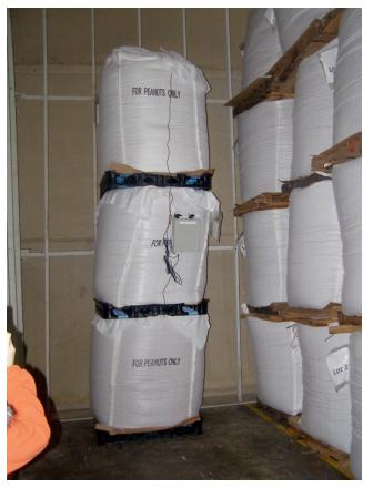
Fig. 3. Totes instrumented with temperature, relative humidity, and leaf wetness sensors stacked in a commercial cold storage facility to determine the effect of storage conditions on the moisture content, water activity, and the occurrence of mold during storage.
