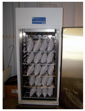
Fig. 2. Placement of samples in controlled environment chamber for studies to determine effect of storage conditions of chemical, sensory, and germination characteristics of shelled peanuts.
