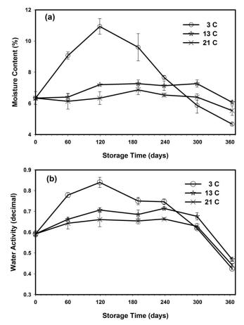
Fig. 6. Average moisture content (a) and water activity (b) of peanut samples retrieved from storage chambers maintained at 3, 13, and 21 C sampled every 60 d for 360 d.
