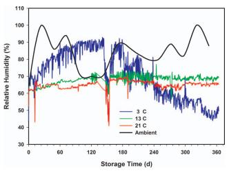
Fig. 5. Relative humidity measured at the Hooks Hanner Environmental Resource Center and in the controlled environment chambers for 360-d storage tests for shelled peanuts.
