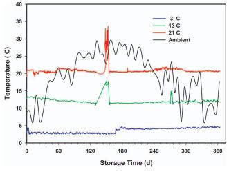
Fig. 4. Temperature measured at the Hooks Hanner Environmental Resource Center and in controlled environment chambers for 360-d storage tests for shelled peanuts.
