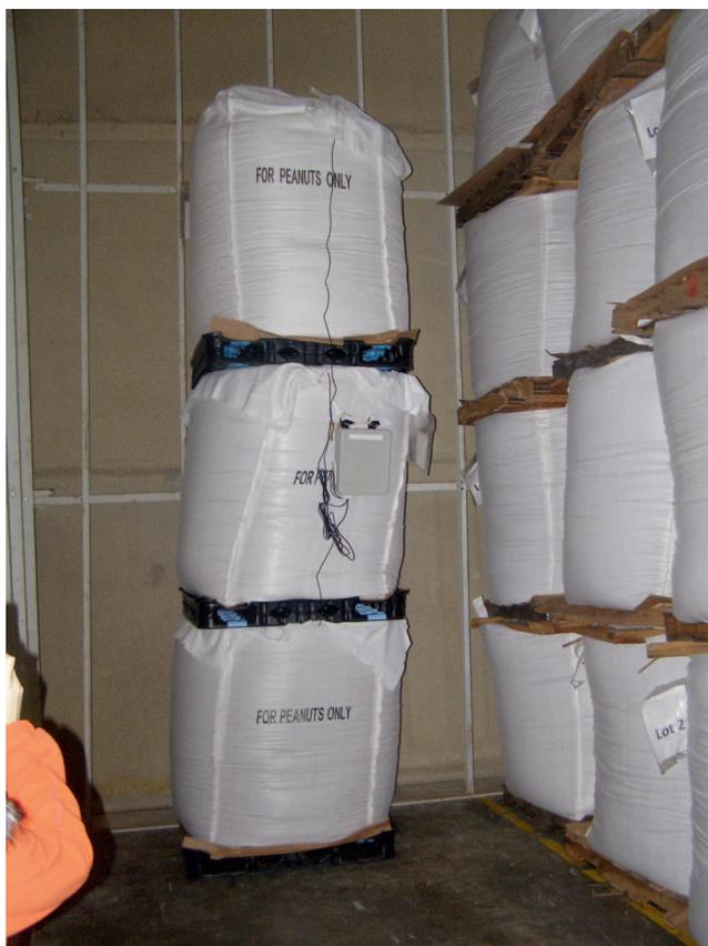
Fig. 3. Totes instrumented with temperature, relative humidity, and leaf wetness sensors stacked in a commercial cold storage facility to determine the effect of storage conditions on the moisture content, water activity, and the occurrence of mold during storage.
