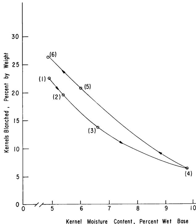
Fig. 3. Effect of Kernel Moisture Content on Peanut Kernels Blanched.
