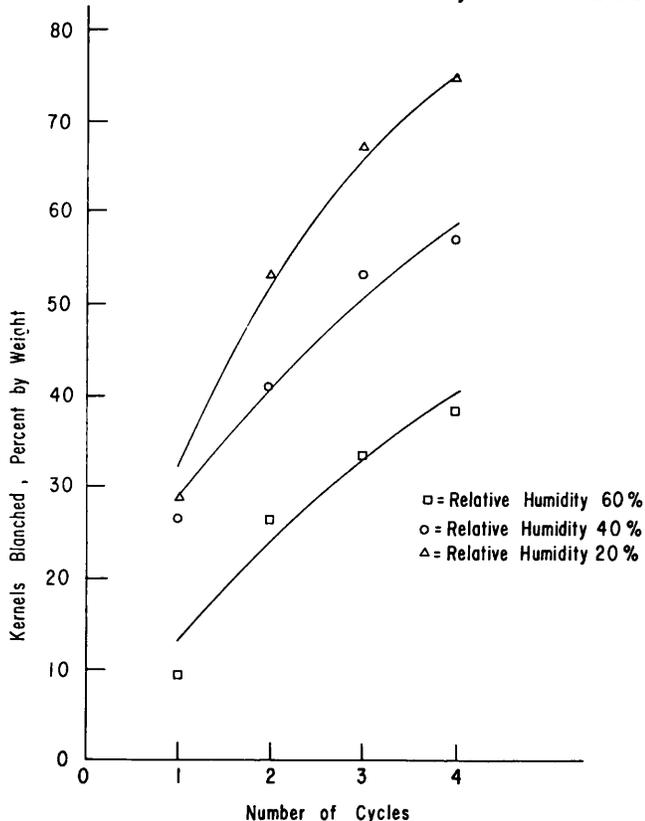
Fig. 1. Effect of Number of Rewetting-Drying Cycles on Peanut Kernels Blanched (Each Point Is the Mean of Three Runs).
