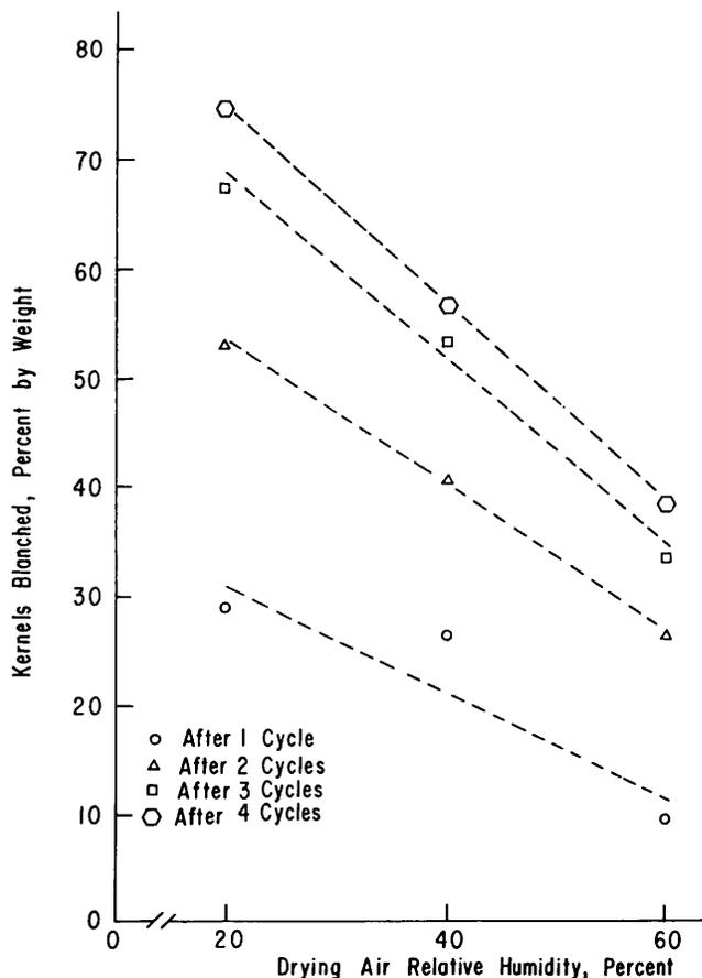
Fig. 2. Effect of Drying Air Humidity on Peanut Kernels Blanched (Each Point is the Mean of Three Runs).
