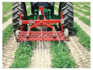
Fig. 1. Photo showing a two-row flexible-tine cultivator in a peanut field.
