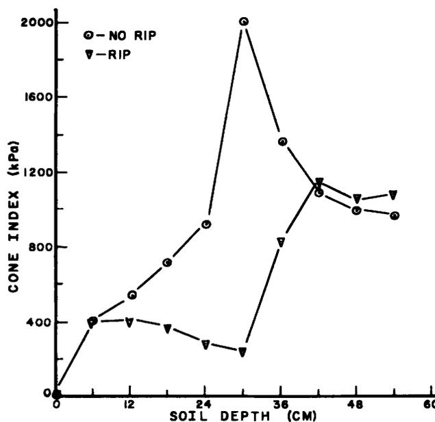
**Fig. 1. Average cone index values with soil depth for no ripping and underrow ripping, 1978, (soil moisture content 10-12% d.b.) Suffolk, VA.****Table 5. The cone index values for different soil depths and seedbed preparations, 1978, Suffolk, VA.**
