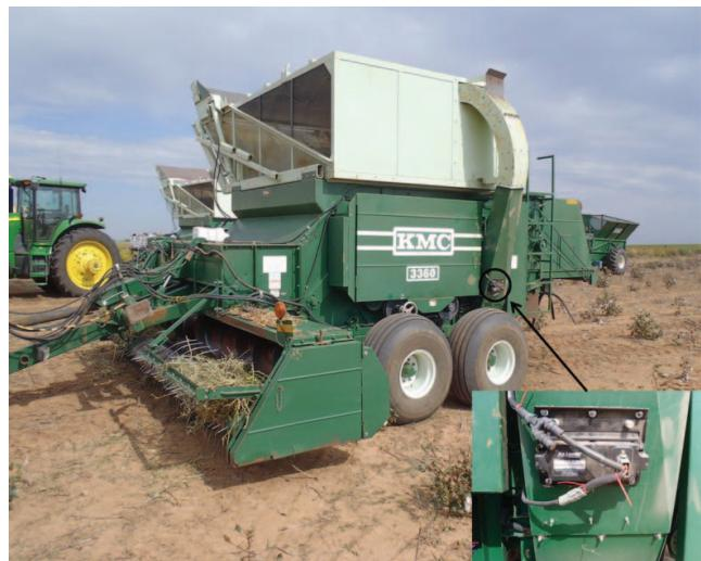
Fig. 1. The mounting location of the AgLeader Yield Monitor on a KMC 6-Row Peanut Combine.
