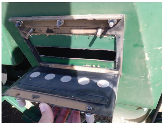
Fig. 3. A representation of the optical sensors after three days of harvest, dust and dirt lightly accumulates, but there is little to no damage due to the deflector plates.
