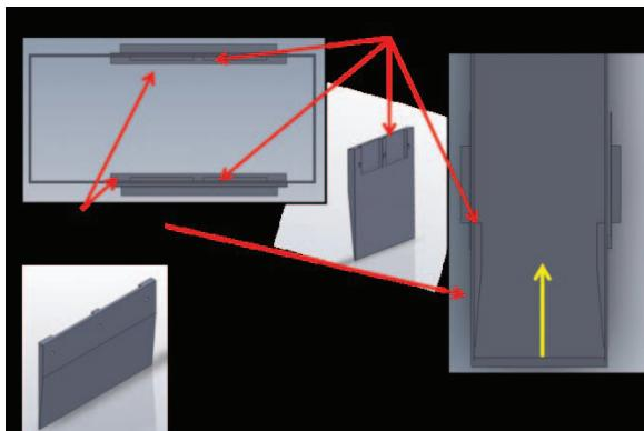
Fig. 2. CAD drawings of the deflector plate mounted inside of the combine chute. From top left clockwise, it is the air vents in the deflector, the back of the vents shown, the vents mounted in the chute and a front view of the deflector.
