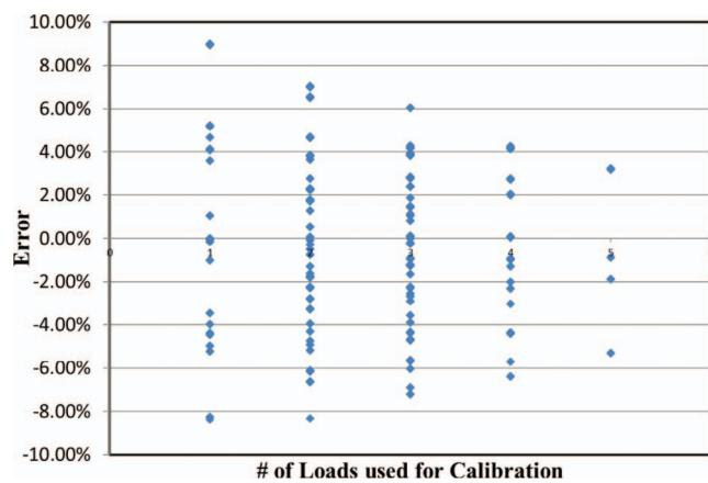
Fig. 5. The graphical representation of the total error and the number of calibration loads applied to the yield monitor, the more calibration loads that were used the total error was reduced.
