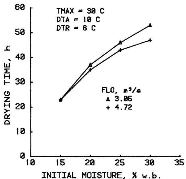
Fig. 3. Effect of airflow rate on drying time.
