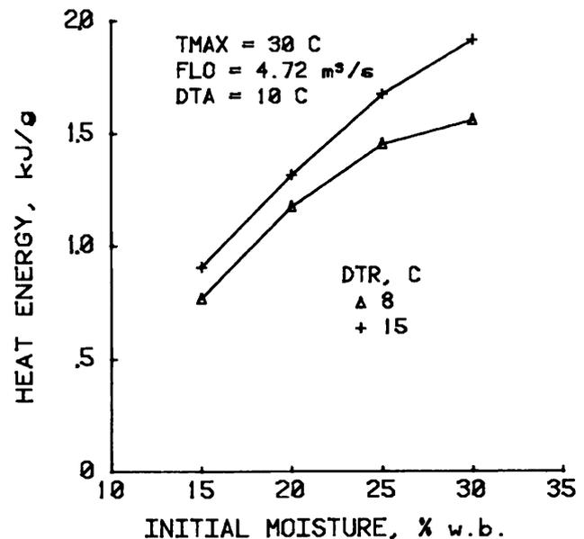
Fig. 6. Effect of drying-air temperature rise on energy use.
