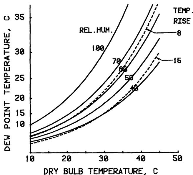
Fig. 1. Relative humidity vs. drying-air temperature rise on psychrometric chart.
