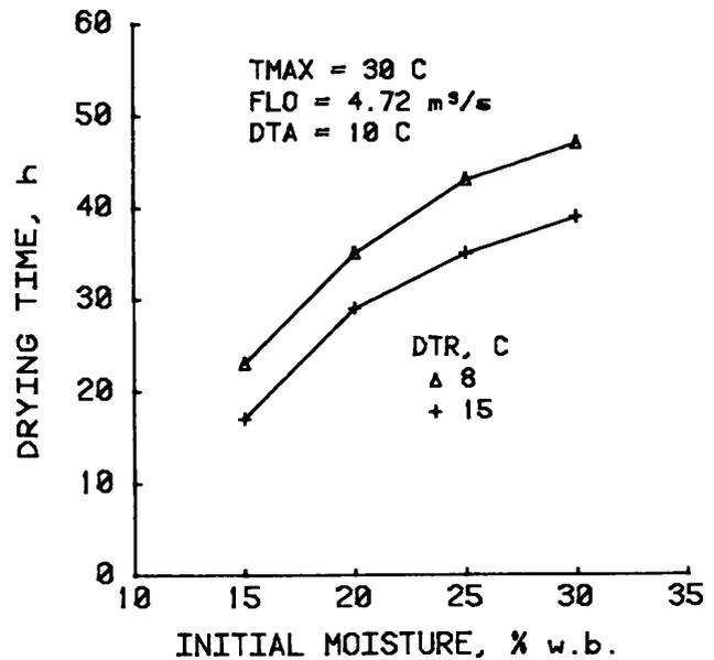
Fig. 5. Effect of drying-air temperature rise on drying time.
