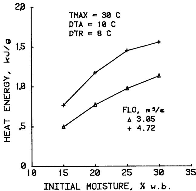
Fig. 4. Effect of airflow rate on energy use.
