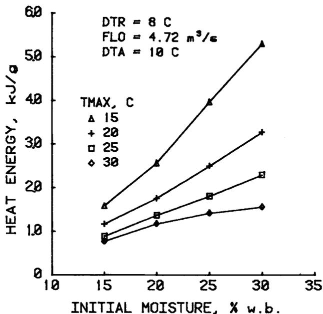
Fig. 7. Effect of maximum ambient temperature on energy use.
