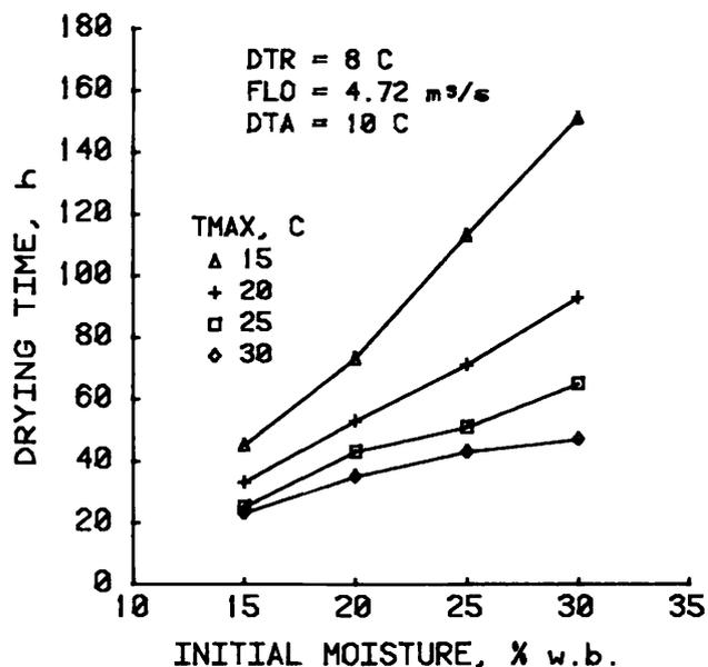
Fig. 8. Effect of maximum ambient temperature on drying time.
